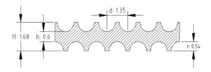
Figure 5.11-2 Individual Lead Foil Profile (Dimensions in mm)
