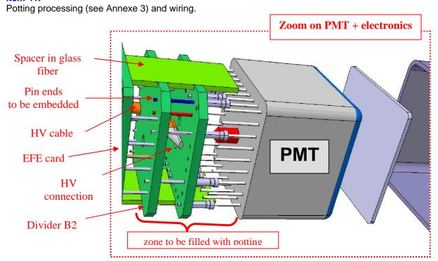
All the HV pins or connections are embedded in DC 93-500 potting. The process as described in the Annexe 3, is an injection of pre-outgassed DC93-500 through a transparent PMT box (visual inspection). Quality check: 1.Visual Inspection during injection (air bubbles), 2. Thermal Vacuum tests for each PMT Tube.
