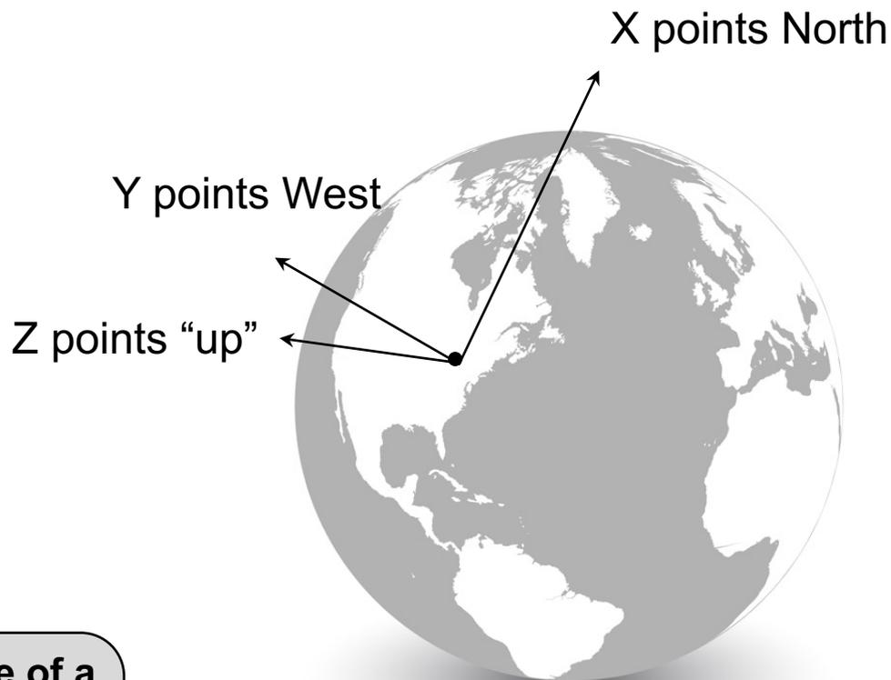
The graphic illustrates one example of a topocentric frame. There is not a standard definition—for example, the z-axis could point down, the x-axis North, and the y-axis East.
