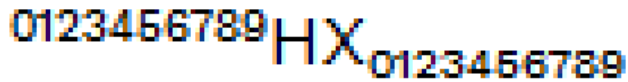
Figure 3.14: For comparison purposes, here the result with option --composites (and no ROUND_XY_TO_GRID ). The composite glyphs as a whole get hinted; consequently, the subscript glyphs get separate blue zones. At the displayed size of 16ppem the vertical positions of the subscript blue zones are rounded differently if compared to the superscript zones, thus the smaller glyph height.
